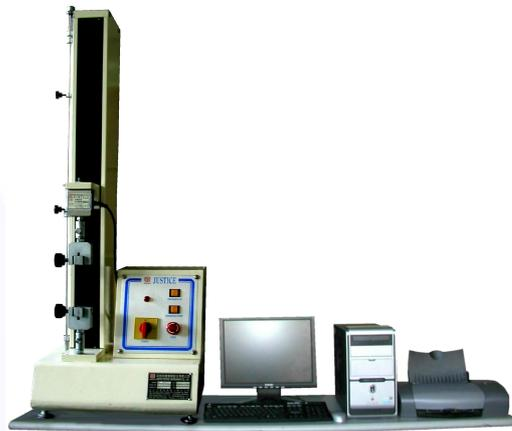
**JIA-803PC 精密型電腦拉力試驗機**
