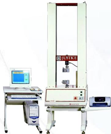
**JIA-802PC 桌上型電腦拉、壓力試驗機**
